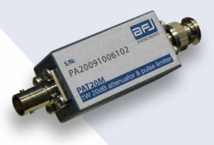
PAT20M Attenuator & Pulse Limiter is designed for pulse voltages up to 1Ws to protect the input stage of EMI receivers with 20dB attenuation.
