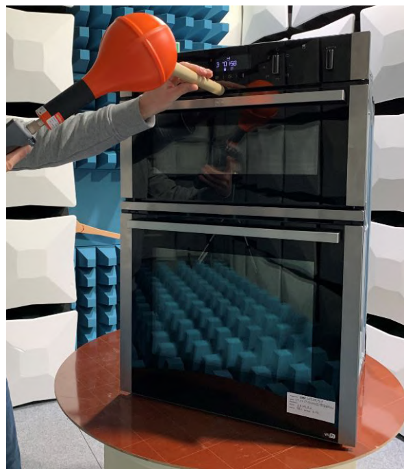
Figure 5: EMF assessment of EUT using the SMP2 in an anechoic chamber.
