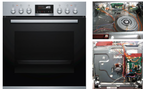
Figure 2: (on the left) Equipment under Test (Commercial Oven with Pyrolytic self-cleaning function), (top right) The top view with cover removed containing cooling fan, user interface and COM2 module; (bottom right) Rear view with cover removed containing hot air fan and control power module.
