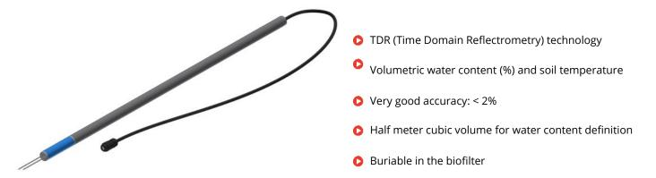
DQA340.1 is the ideal solution for the measurement of temperature and volumetric moisture (0-100%) in biofilters. The sensor is based on TDR technology (Time Domain Reflectometry), ensuring good accuracy even in very wet soil. Using its plastic shaft, the sensor can be inserted in the material.
