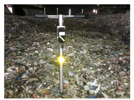
EXP sensors range has been specially designed for their application in industrial composting plants, waste treatment plants and wherever the environmental conditions are severe. Comparing to most of the similar sensors on the market, EXP sensors are designed for monitoring applications, where the sensor need to measure non stop for several weeks.
